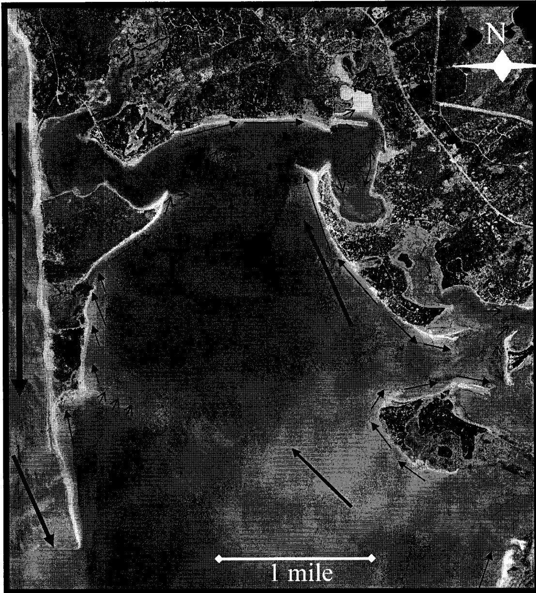
Figure 3.18: Sediment transport map of Wellfleet Harbor that shows the dominant direction of transport is from Cape Cod Bay up into the Harbor and Herring River.
