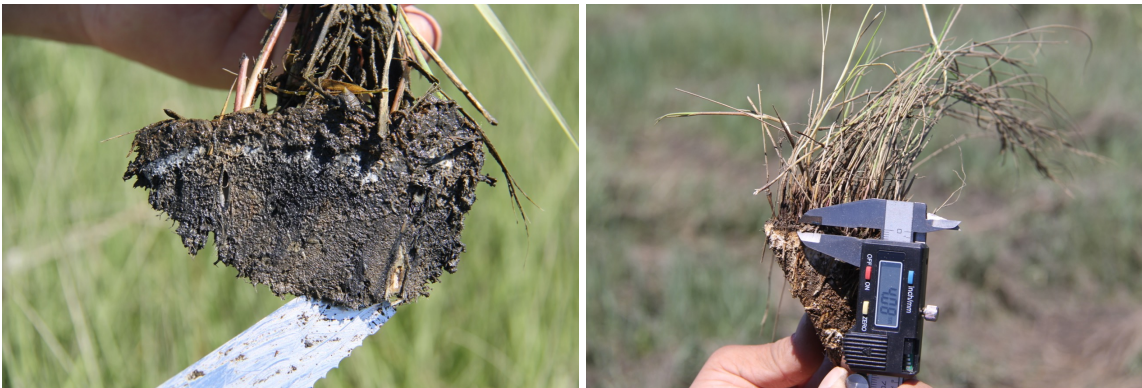
Figure 10. Examples of sediment accretion in low marsh creek bank (left) and high marsh (right) marker horizon plots.
